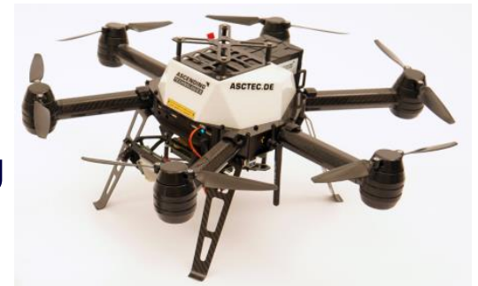
MAV with embedded CPU
